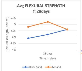
M sand can be effectively used in Construction As a replacement of River Sand. And to preserve the Water bodies for future, and to Promote the Eco-friendly construction processes.
